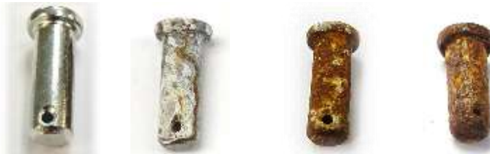
1. New bolt 2. Acceptable 3. Replace 4. NOT acceptable
